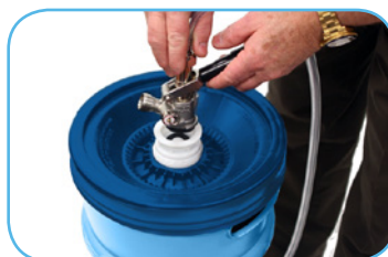
2. When the keg is without pressure, disengage tap by pulling out, up, and twisting the handle
