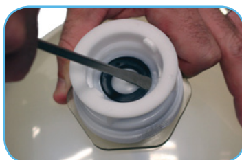
5. To relieve additional pressure in the keg, create an air gap by carefully opening the seal between the rubber cap and the valve body with a tool similar to a flat head screw driver
